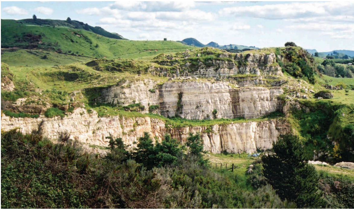
Figure 2. Thin bedded zeolitic tuffs exposed over a thickness of about 30 m in quarry benches at the Mangatete Road zeolite deposit.
