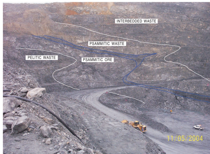
Figure 1: The complex geology of the HMSZ, outlining the hanging wall bounded by massive psammites in the north wall of Frasers 3 Pit.
