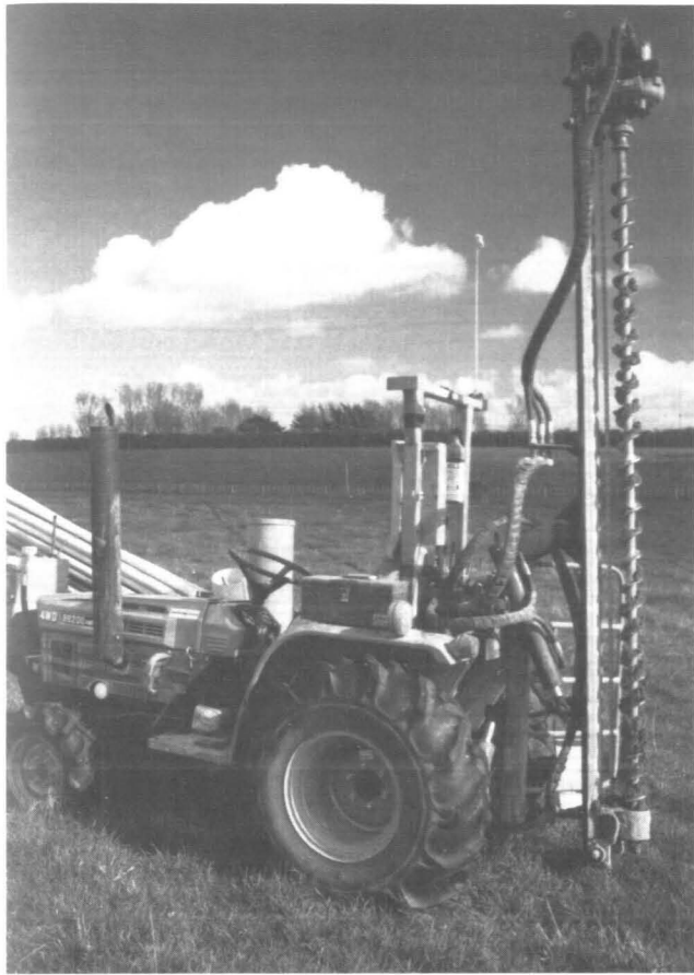
Figs. 10a and b: Hydraulic auger drill mounted on Kubota 4x4 tractor.
