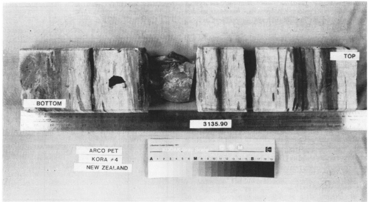
Figure 7: Interbedded burrowed, glauconitic marlstone and dark gray claystone comprising Unit 4 at 3135.4-3135.9 m. Burrows are primarily horizontal and occur in the greenish-gray marlstone. Burrow types in Unit 4 include Zoophycos (arrow), Thalassinoides , Teichichnus , and Chondrites .
