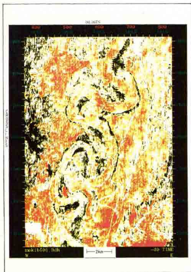
Fig. 11. Seiscrop display above the mapped Moki B5 event showing a meandering channel complex at top Moki B Sand level (detail from northern Maui PML).
