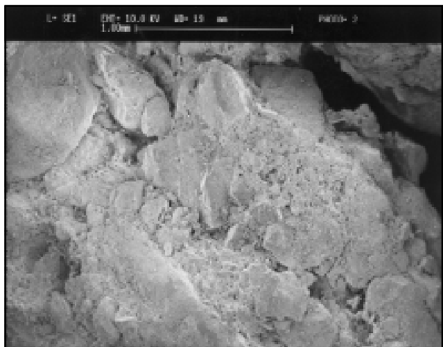
Figure 12a: Typical SEM view of the Kawau Sandstone from Hoiho-1C.
