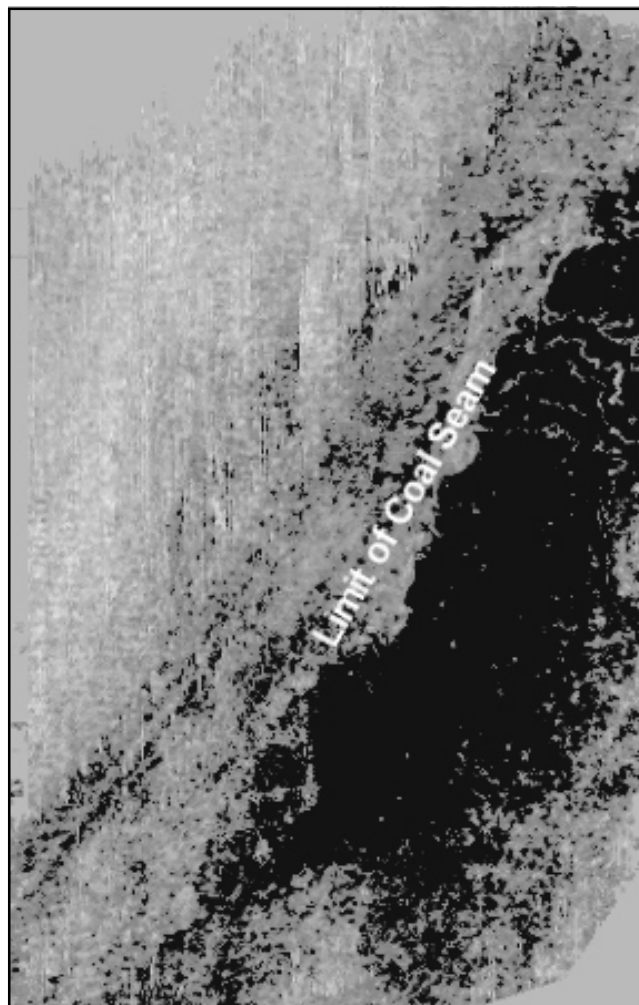
Figure 10: Seismic TWT slice showing the limit of a coal seam within the Mangahewa area.
