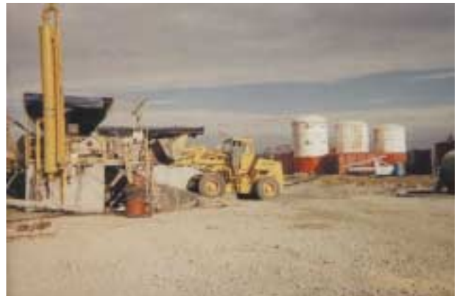
Figure 9: Mobile liquid mud plant.
