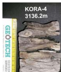
Fig 8. Coal and shale clasts in Tangaroa sandstone core samples
