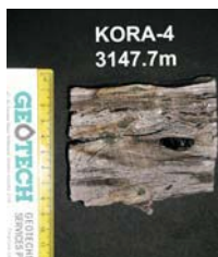
Fig 7. Coal and shale clasts in Tangaroa sandstone core samples
