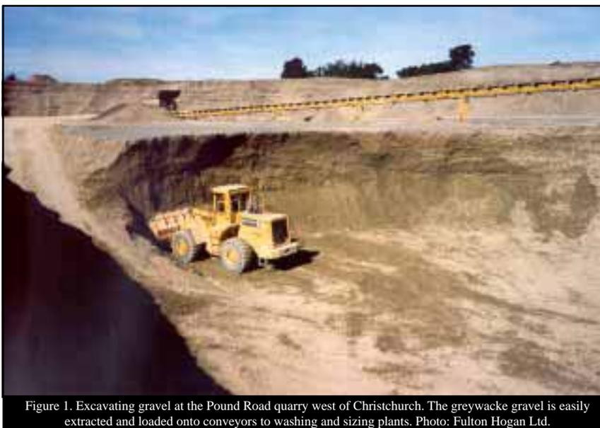
Figure 1. Excavating gravel at the Pound Road quarry west of Christchurch. The greywacke gravel is easily extracted and loaded onto conveyors to washing and sizing plants. Photo: Fulton Hogan Ltd.
