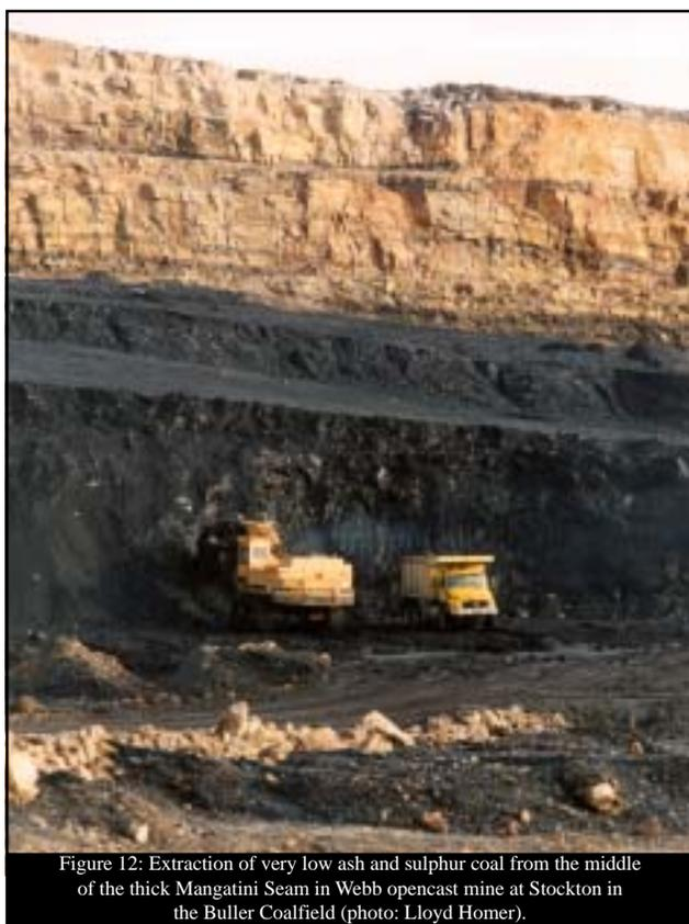
Figure 12: Extraction of very low ash and sulphur coal from the middle of the thick Mangatini Seam in Webb opencast mine at Stockton in the Buller Coalfield (photo: Lloyd Homer).
