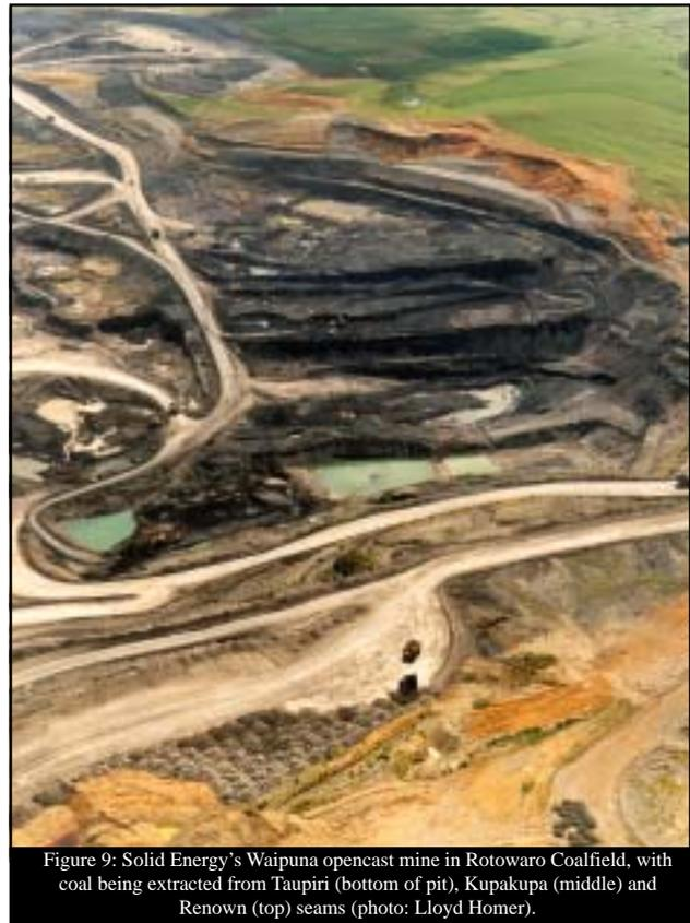
Figure 9: Solid Energy's Waipuna opencast mine in Rotowaro Coalfield, with coal being extracted from Taupiri (bottom of pit), Kupakupa (middle) and Renown (top) seams (photo: Lloyd Homer).
