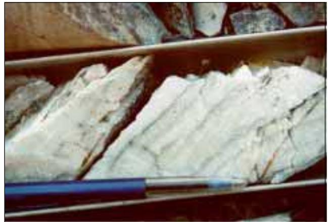
Figure 2: Banded quartz of the Birthday Reef in hole WA11A at Blackwater (Waiuta), drilled by Macraes Mining in late 1996 (Photo: Tony Christie).
