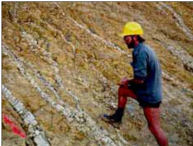
Figure 10: Narrow quartz veins that lie between the Welcome and Martha veins (not shown), exposed in the southwestern pit wall of the Martha Hill mine (Photo: Tony Christie).
