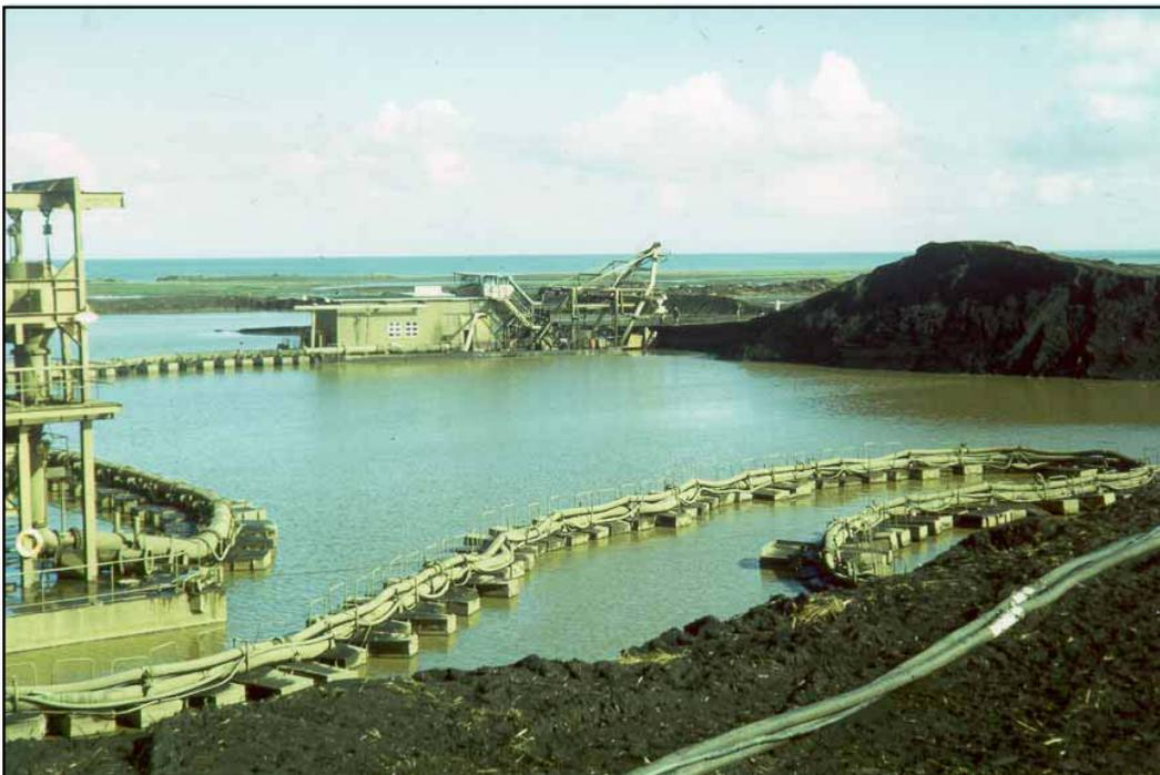
*Figure 6: Ironsand dredge and floating concentrating plant at the former Waipipi mine, near Waverley (Photo: Bruce Thompson).*
